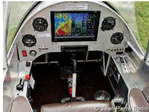
Flaps are electrically continuous, 35 degrees worth, with a nifty indicator on the right subpanel. Four steam gauges provide backup to the Dynon; VSI, altimeter, ASI and turn and bank, right to left.
